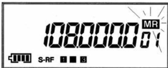
Change the memory frequency stored within the memory location by pressing the up or down button to select the desired frequency.
