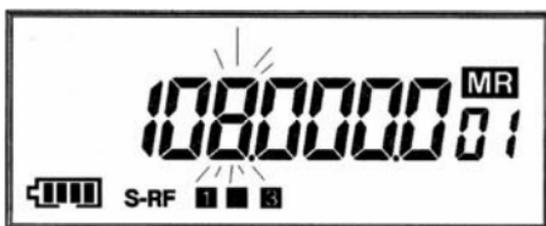
When frequency selection has been made, to store in to memory, press the MR (MW) or "MON" button.
